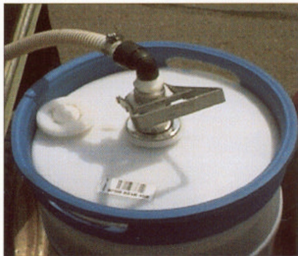
Returnable, refillable containers and closed-system pump offer convenience and safer handling of materials.
